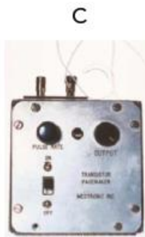
Earl Bakken and C. Walton Lillehei create a battery-powered external pacemaker
