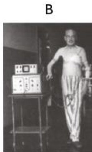
AC-powered pacemaker units attached to an extension cord
